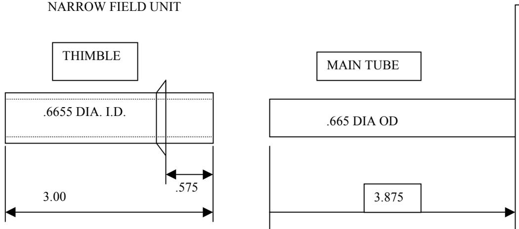
THESE UNITS HAVE THE SAME FOCUS ROD THREAD AND LOCATION, OFF AXIS AS CURRENT UNITS. THIS LOCATION IS 15/16 DOWN FROM OPTICAL AXIS AND .500 OVER. A CONICAL SPRING WAS LOCATED ON AXIS IN MOST UNITS AROUND THE MAIN TUBE.
