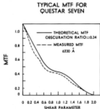
Typical Questar Seven Modulation Transfer Function (MTF) as obtained with a shearing interferometer and expressed as a function of the shear parameter, S. To express the MTF as a function of the spatial frequency, R, in lines per millimeter, the following relationship can be used:
